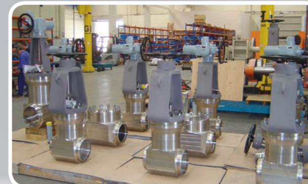
Gate & Check valves for the Residual Heat Removal System at Ringhals NPP (Sweden).
