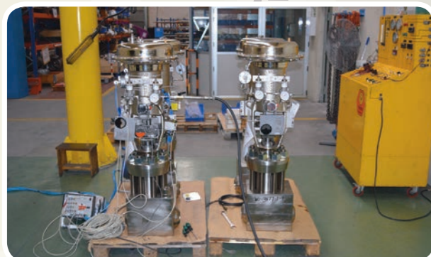
Diagnosis test performed at RINGO premises for Control Valves.
